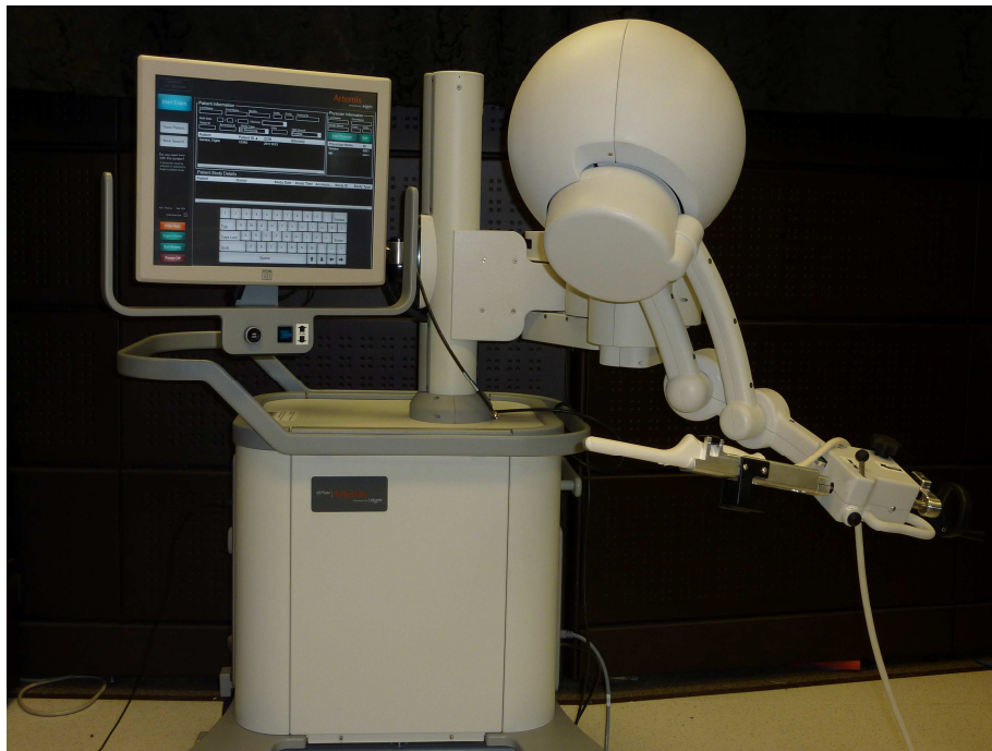
Figure 6.1: Photograph of the Atremis prostate biopsy tracking system by Eigen (Grass Valley, CA).
