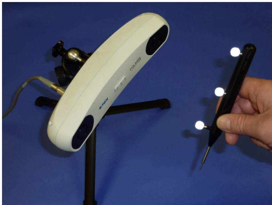
Figure 1.1: Photograph of an infrared optical tracking system from Northern Digital. The three optical markers attached to the tool are imaged from two different angles to determine its position.
